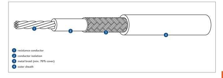
Resistance conductor: Conductor isolation: Metal braid: Min. 70% cover:
