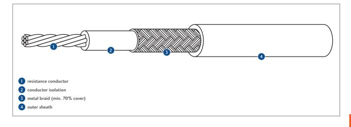
Resistance conductor: Conductor isolation: Metal braid: Outer sheath: see table next page PFA, wall thickn. 0.90 mm (<sup>1)</sup> 1.00 mm) Cu-nickel-plated 16 x 5 x 0.15, cross section 1.41 mm<sup>2</sup> PFA, wall thickn.: 0.40 mm (<sup>4)</sup> 0.70 mm) (<sup>5)</sup> 0.80 mm)
