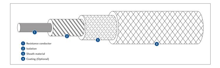
Resistance conductor: Isolation: Sheath material:
